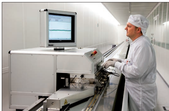
30 m long measuring machine for scale tapes
