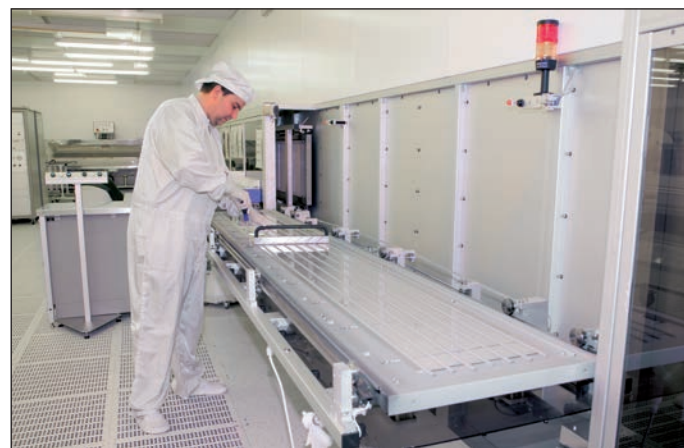
Vacuum machine for application of chromium layers
