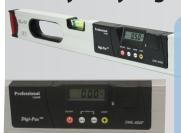
DWL 600 advanced electronic modules, with a resolution of 0.05°, is designed to be fitted into rugged aluminium structure of 600mm length to meet most challenging heavy duty applications. Calibration certificates obtained from USA, Japan, UK & Germany on product specification conformance are available for reference.
