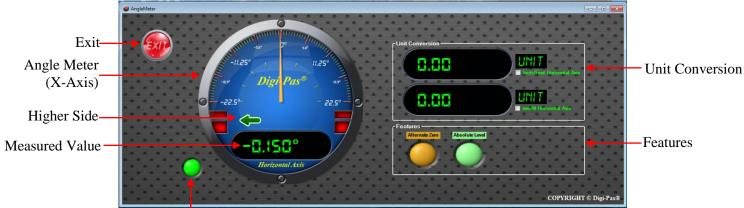
Blinking indicates measurement is in progress
