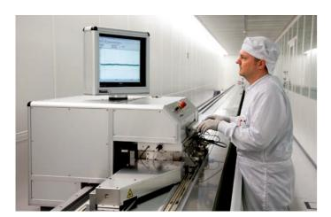
30 m long measuring machine for scale tapes
