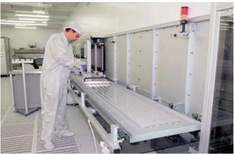
Vacuum machine for application of chromium layers
